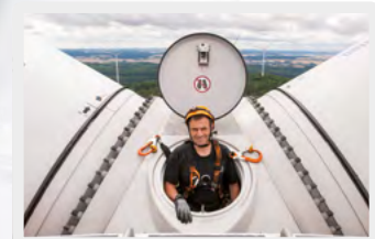
The technicians enter the hub via the roof of the nacelle.
